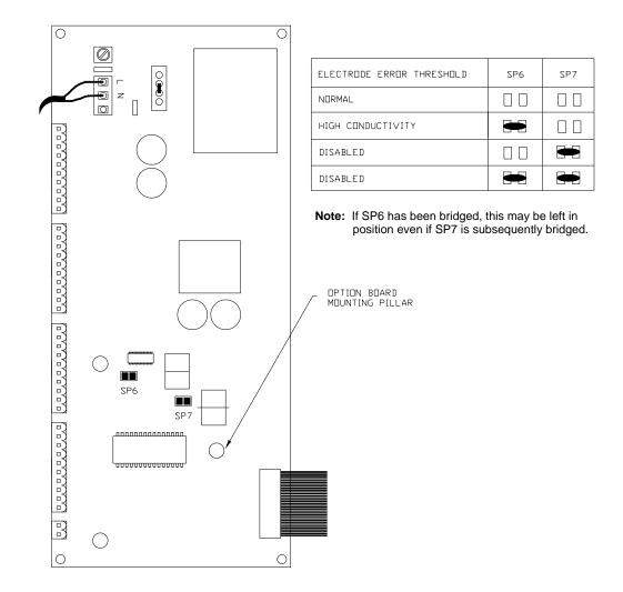
Input Board (Option Board Removed)
